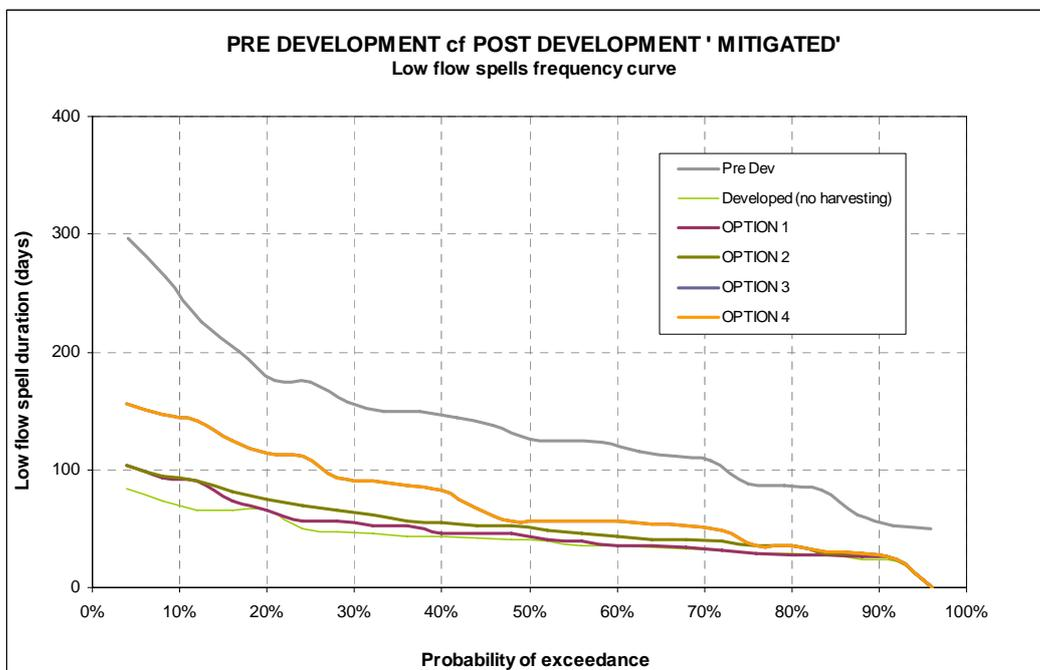
**Figure 2 Low flow spells frequency curves for example stormwater harvesting project**
