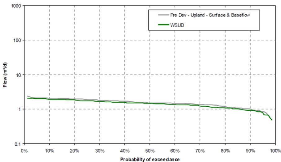
**Figure 4: Low flow frequency duration curve for the same typical Wyong catchment with implementation of the Porters Creek stormwater harvesting scheme**
