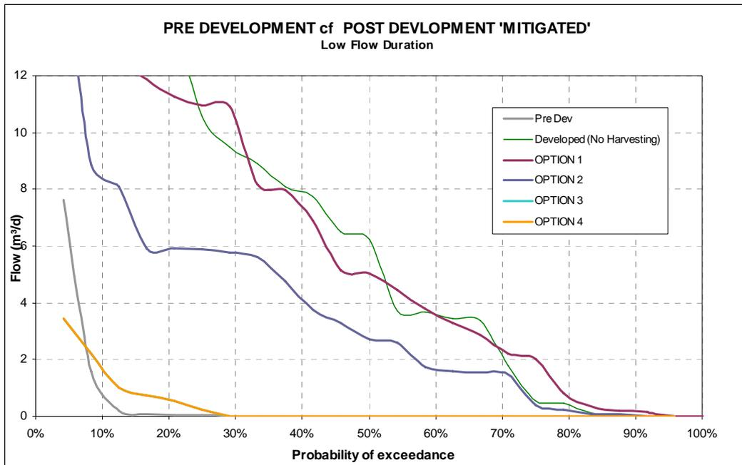
**Figure 1 Low flow duration frequency curves for example stormwater harvesting project**
