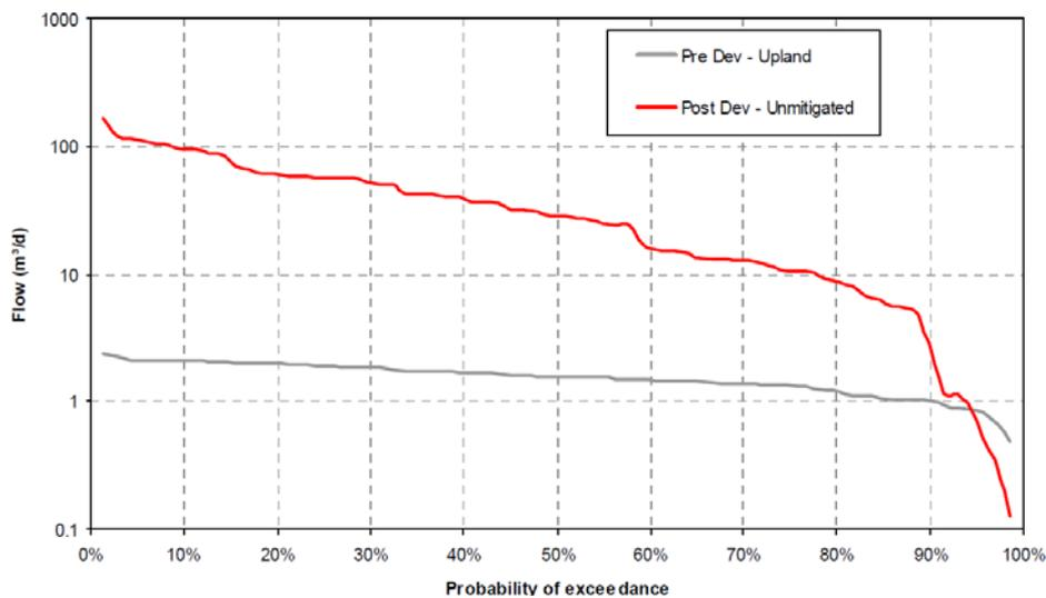
**Figure 3: Example low flow duration frequency curve for a typical Wyong catchment before and after development**
