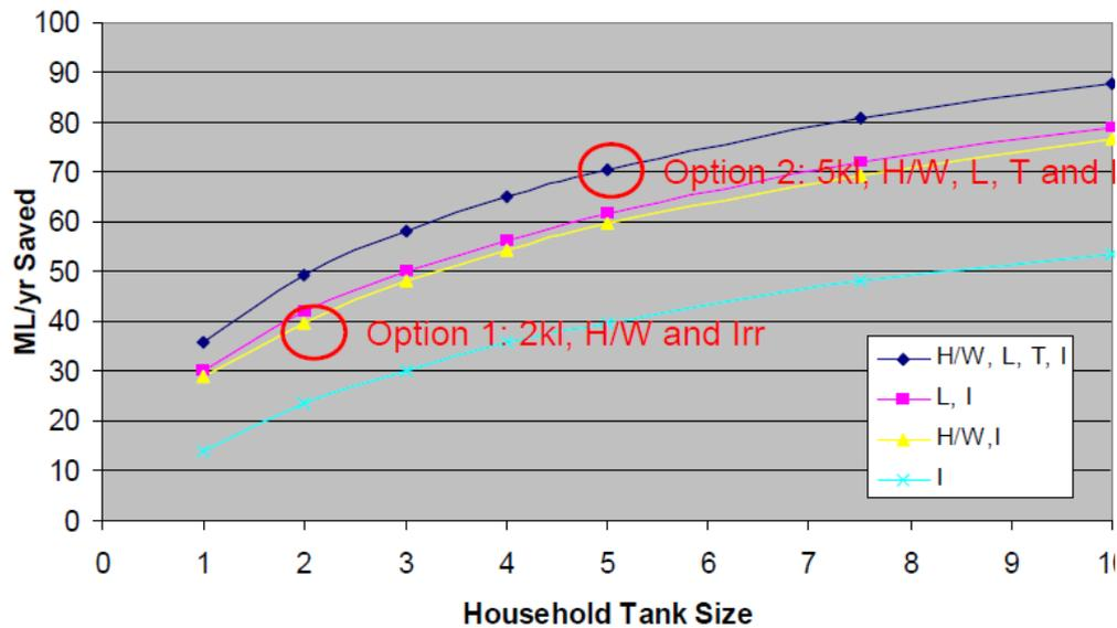
Figure 7: Rainwater tank savings in Lofberg Quarry Creek Catchment
