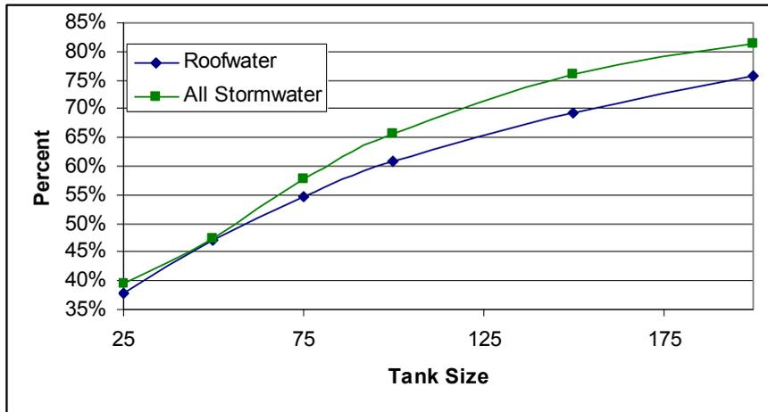
The fourth option would be to collect half the light greywater for toilet flushing and use a smaller rainwater tank for the cold water in the washing machine. A smaller tank size of 25 to 50 kL would allow a further reduction of 5 to 6% (i.e. ~38% of laundry demand) on the 15% saved by reusing greywater for toilet flushing. This would be a combined water saving of approximately 50% for the
