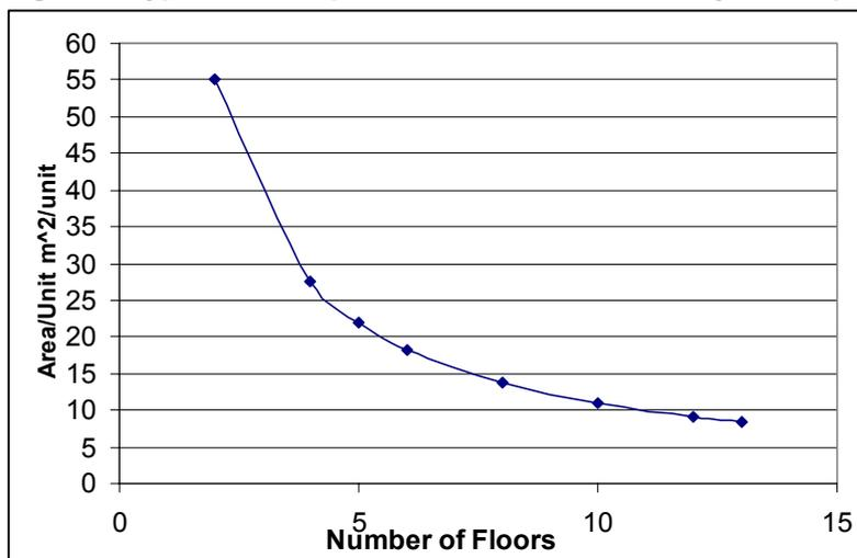
A typical ratio of roof area to number of floors and the ratio that has been used for this analysis is shown in Figure 3. As the number of floors increase, the roof area per unit decreases substantially.
