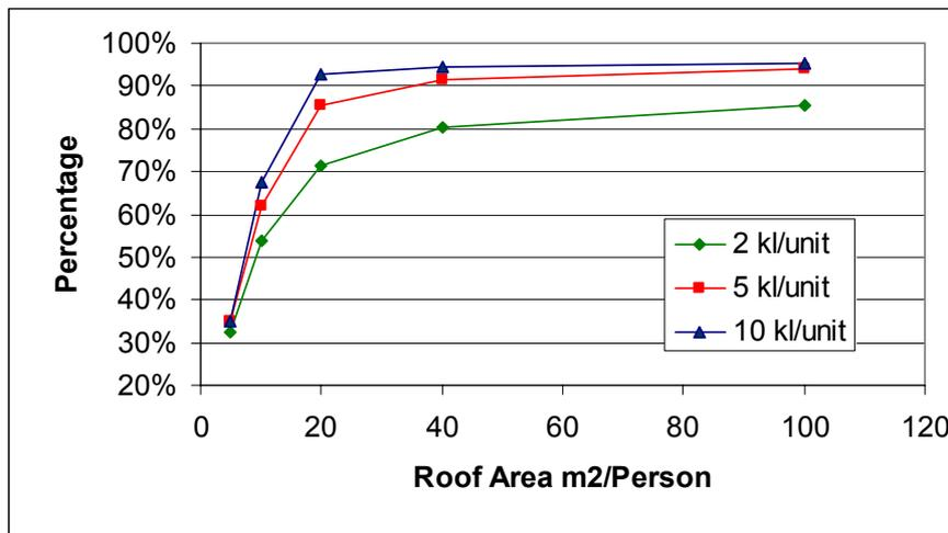
At about 20m<sup>2</sup> of roof area per person and above however there is a clear difference in plumbing water into laundry and toilets. For the relatively small extra cost of plumbing into the laundry facilities, potable water consumption reduces by a further 10 L/d for a 2kL/unit storage and about 15 l/d for a 5 and 10 kL storage per unit. Figure 6 also shows that there is little advantage in going above 5 kL/unit of storage per
