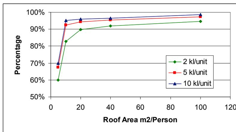
Figure 5 shows a similar analysis reusing harvested roofwater for toilet flushing and cold water laundry washing. The cutoff limit for sizing a roofwater storage is about 5 kL/unit.
