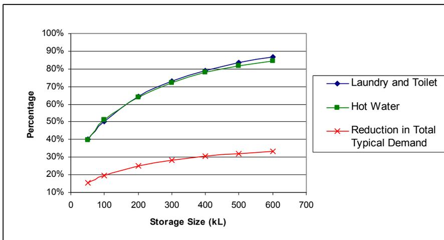
Analysing option 2 for optimum sizes shows that an optimum storage size for both treated stormwater and roof water is about 100 to 200 kL. This will give a reduction in potable water compared to a typical dwelling of about 20 to 25%. This development with water efficient fixtures would exceed the BASIX requirement of a 40% reduction, not including
