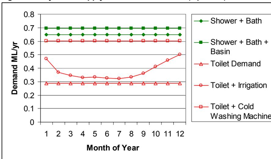
An analysis of option 3 shows that there is an excess of light greywater (wastewater from the shower and bath and basin) compared to the demand for the toilet and irrigation use on site. If the majority of the shower and bathwater is collected and reused for toilet and irrigation demand on the site then an additional 15% reuse can be achieved. This option would meet the
